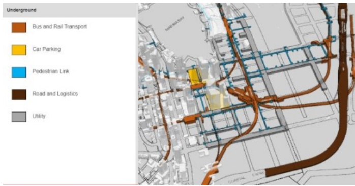
The 3D Underground Space Plan shows specific locations of underground infrastructure, including rail networks, utilities and pedestrian links
