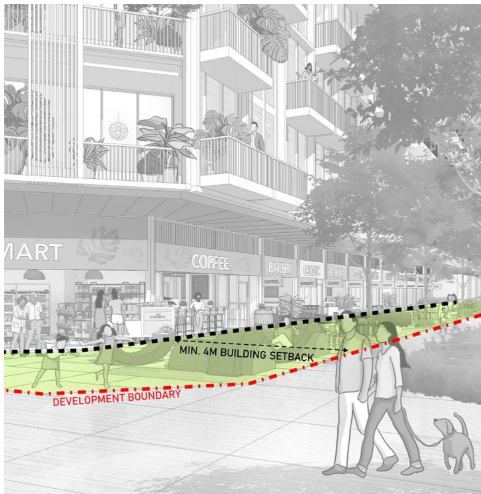
Example of building setback for the Neighbourhood Street along Marina South Avenue Marina South Urban Design Guide
