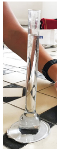
Left: Karsten Tube test on encaustic tile to assess water absorption rate by capillary action.
