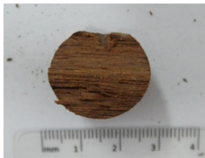
Extracted sample of a historic timber element for microscopic study.
