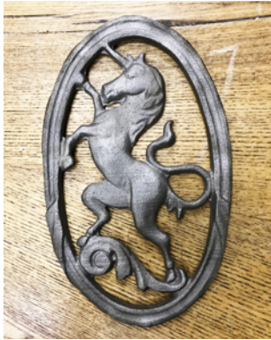
Cast-iron unicorn motif 3D test print replica using metal powder as printing medium, produced from 3D scanning data.
