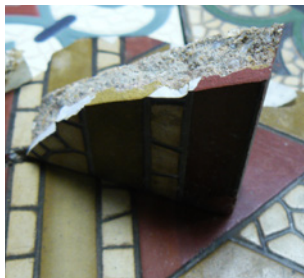
Polychromatic cement tile fragment showing pigmented finishing layer on a 'body' of grey Portland cement. Grooved imprints are added for slip resistance.
