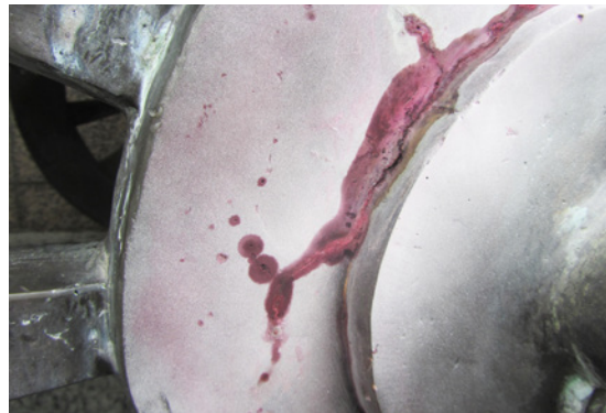
Dye penetrant test highlights presence of cracks and pitting on metal.
