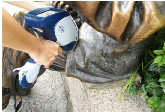
Portable XRF used for in situ elemental identification.
