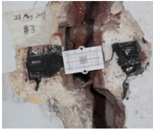
Avongard Tell-Tale crack gauge for monitoring changes in crack widths.
