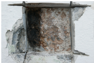
Sampling for investigation can be invasive, commonly requiring controlled 'breakouts' and drilling of materials for processing in the lab.
