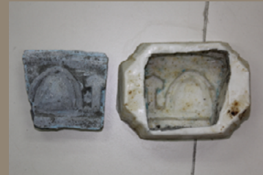
LEFT: A profile gauge for recording simple profiles on cornices. ABOVE: Replica created from a silicone mould.
