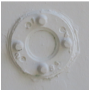
Attached permanently to the side of historic buildings, a tilt plate provides a constant point from which measurements can be taken, using a separate handheld device. Changes are found by comparing the current reading to the previous recorded reading.
