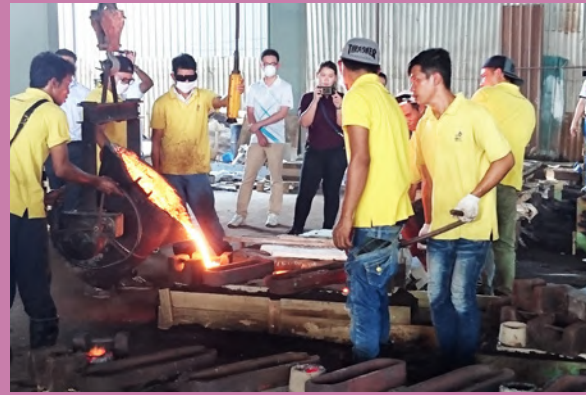
Molten iron being poured into a mould to recast rainwater gutters.
