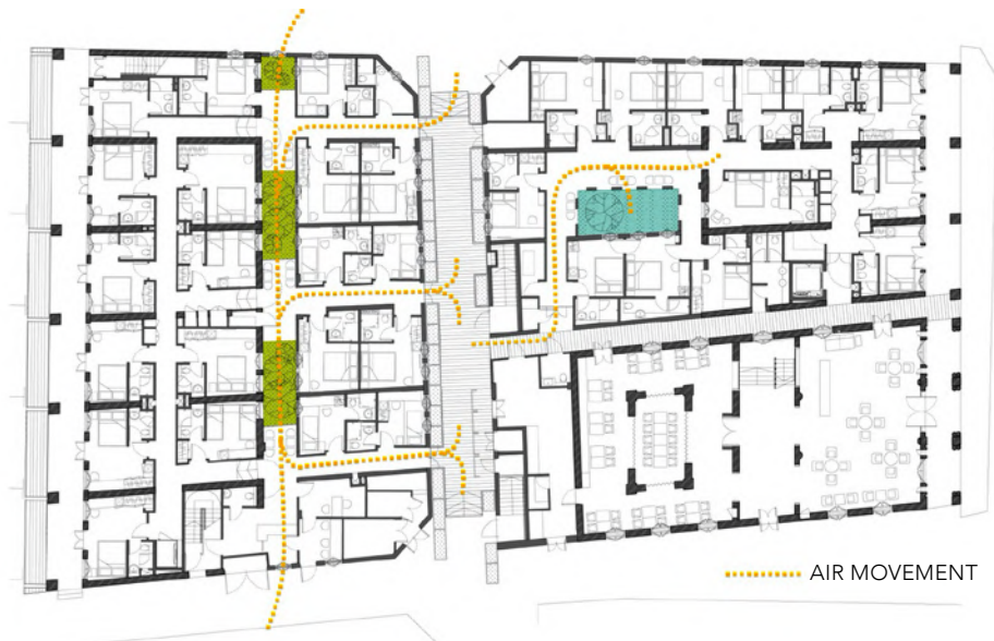
Air movement through the hotel is facilitated by the new courtyards and natural ventilation.
