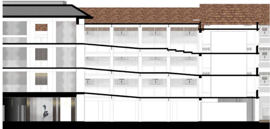
Left: Elevation outside the newly added corridors (on the left) subtly contrasts with the adjacent and opposite historic corridors. Right: Schematic section depicts introduction of accessibility-compliant ramps to offset level differences.
