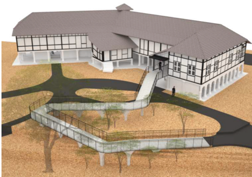
A delicate new entrance ramp added at the rear of Atbara provides universal access and maintains the visual integrity of the building's historic front
