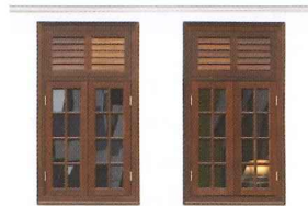
Casement windows of shophouses
