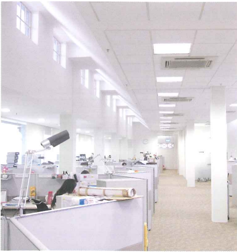
Specially designed ceiling profile to bring in natural lighting
